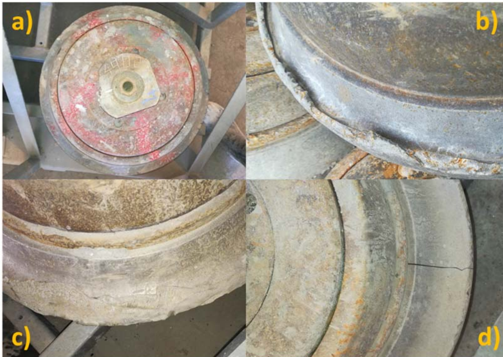
Figure 30 Illustration of the reasons for replacement of cutter rings a) Abrasive wear, b) Mushrooming, c) Chipping and d) Ring crack.
