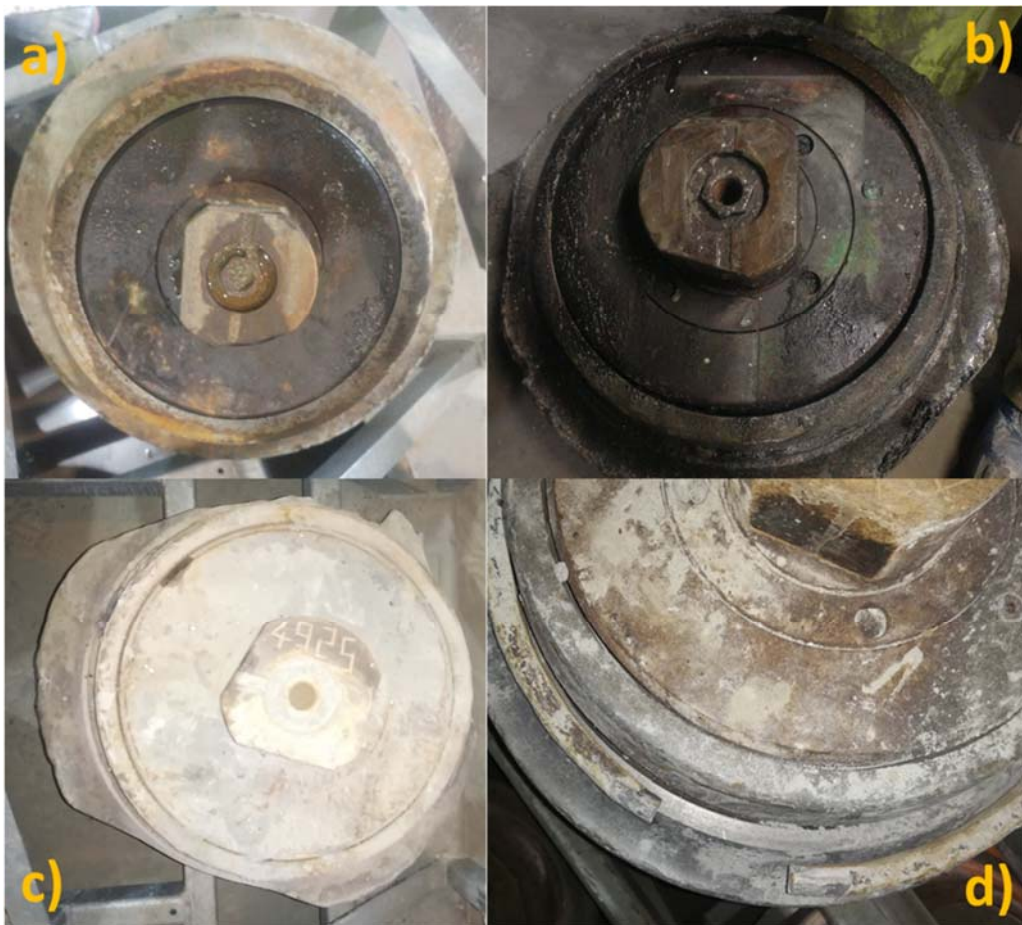
Figure 31 Illustration of the reasons for replacement of cutter bearings a) Oil leakage, b) Oil leakage with indication of blockage, c) Blocked cutter and d) Other reasons (including cracking).
