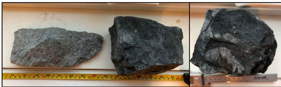
Figure 28 Example of chips of Gneiss (left) and Amphibolite from the same chipping analysis (i.e., from the same tunnel face). (Photo: Javier Macias).
